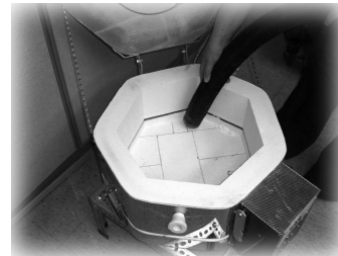
Vacuum any loose debris
