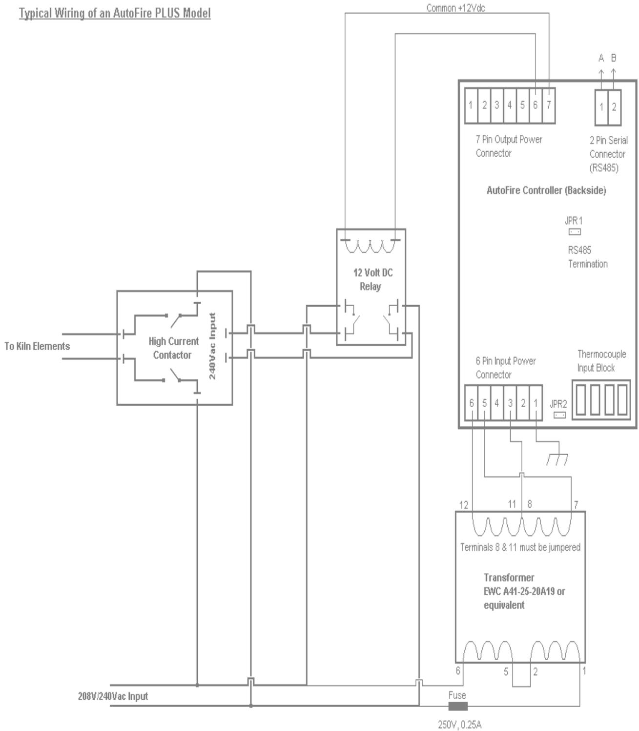
**Typical Wiring For A AutoFire Plus or UniTemp Model**
