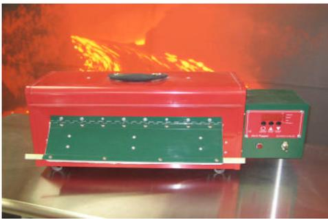
It is important to have an air space under the kiln. If you have a wood table or a wood table with a metal top, you need to put smooth ceramic tiles down first. You can cut a piece of dry wall or cement board larger than the tool box base and put it down as base. To clean up the look use a strip of duct tape around the edges of the dry wall. Call with any questions. 863-648-0585
