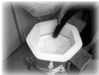
Vacuum any loose debris
