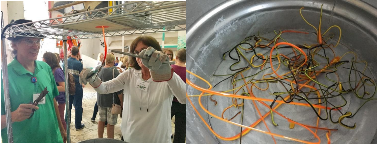
Shown above is a slow pull with tweezers and a helper to cut the glass! Work slowly and safely.
